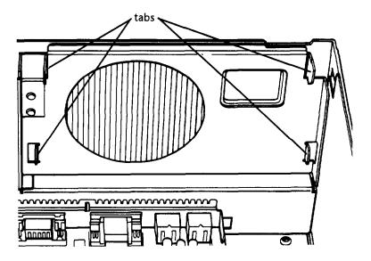
Lift up the subassembly from your work surface and lower the back end into the computer, fitting the top tabs in the computer into the openings in the top slots on the subassembly.
